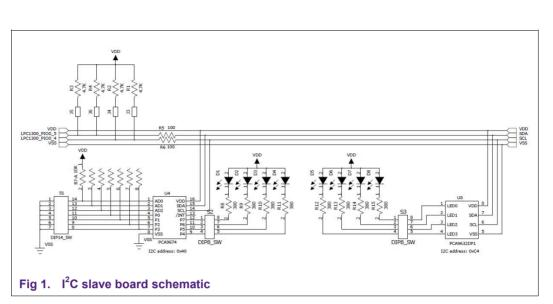
S1.1~S1.3 are the address selectors for the PCA9674. Setting all switches to ON will configure the PCA9674 address as 0x40.
