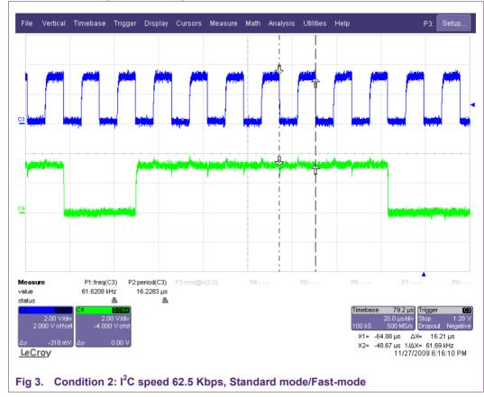
2.2.3.2 Condition 2: I<sup>2</sup>C speed 62.5 Kbps, Standard mode/Fast-mode
