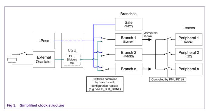
To save power it is essential that as little logic is working as possible. Figure 2 illustrates a simplified clock structure that makes it easy to see how the switches need to be configured.
